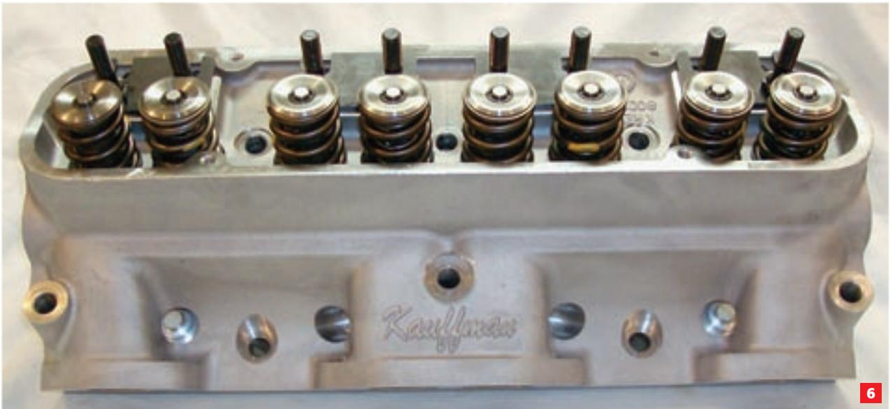
**6 In fully-assembled form, the heads are ready to bolt on. The stud girdle kit is available as an option, but is recommended.**
