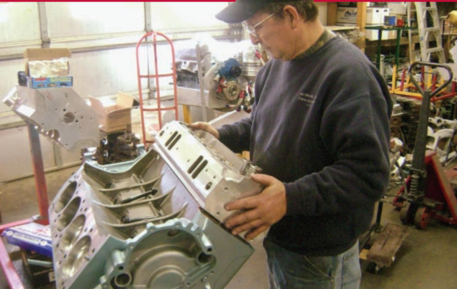
By raising the intake ports on their High-Port heads, Kauffman Racing Equipment was able to straighten out the intake port and dramatically improve airflow to the back of the valve. Better flow is essential to making power, and these heads can flow: how's 630- horses on a pump-gas 467-inch Pontiac sound to you?
