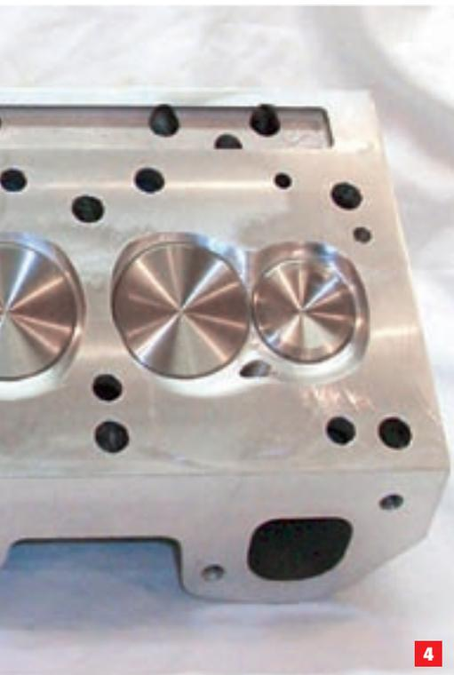
**4** The High-Port heads are available in several different chamber sizes to meet your target compression goals. Again, the chambers are fully CNC-machined and the valves are Ferrea 1200 series 2.20/1.70-inch pieces, and the spark plug angles are slightly revised. Note the exhaust ports, which are based on standard Pontiac port configurations to minimize exhaust system mating hassles.
